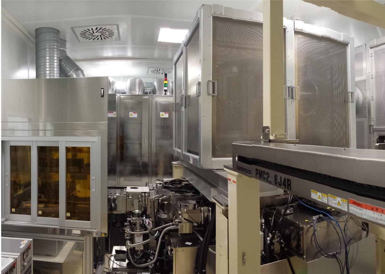
Multi-Beam Column on air-bearing Stage Platform
