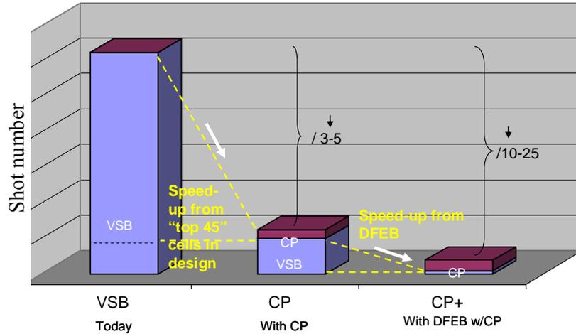
Figure 3 : Shots number reduction perspective using a standard cell projection lithography and an optimised Design For EBeam (DFEB) approach.
