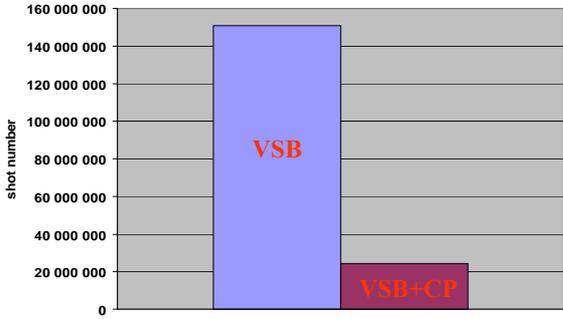
Figure 9 : Shot reduction obtained with Cell projection applied to the 65nm PROMO contact level
