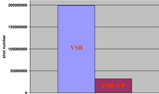
Figure 10 : Shot reduction obtained with cell projection applied to the 45nm PROMO contact level
