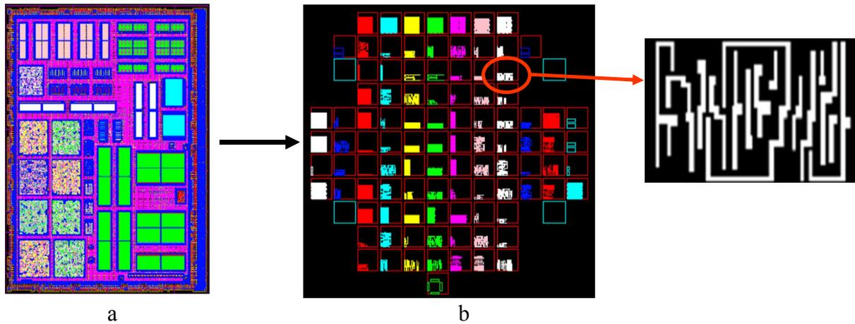
Figure 4: Cells extraction from 65nm memory cells GDSII file (a) and cells placement on stencil mask (b)
