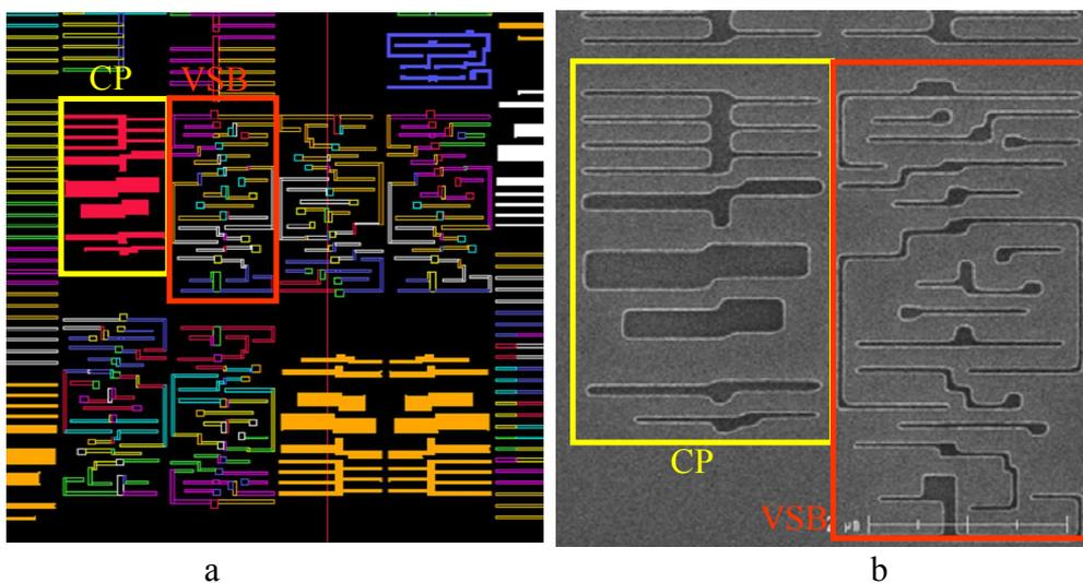
Figure 5 : Example of a data base having the CP and VSB shots (a) and the results on wafer (65nm line width) (b)
