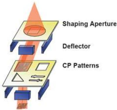
Figure 1 : Illustration of Advantest F3000 cell projection (CP) concept
