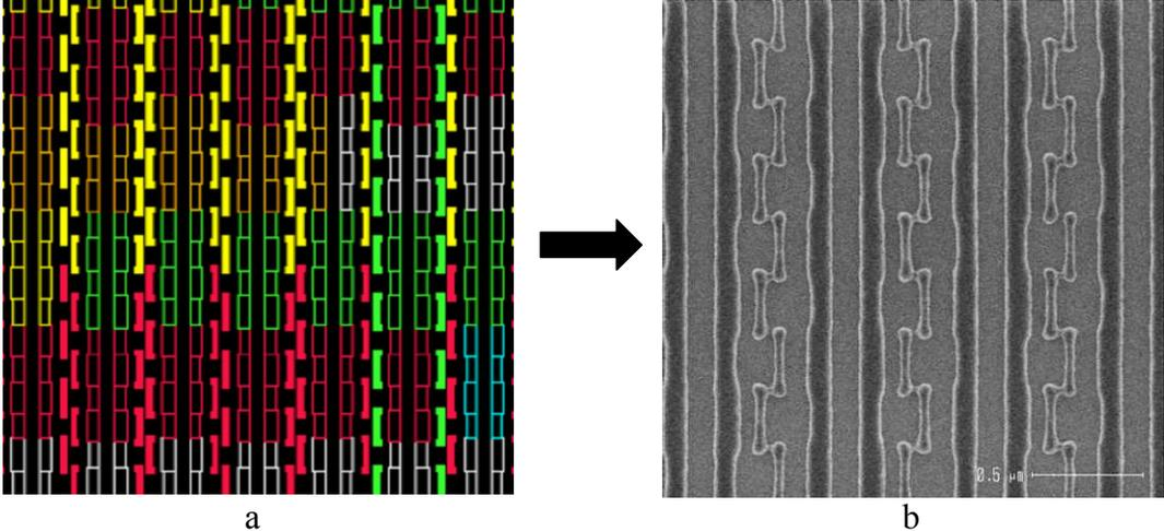
Figure 7 : 45nm SRAM structures active level patterned at 44nm line width with a 85nm pitch
