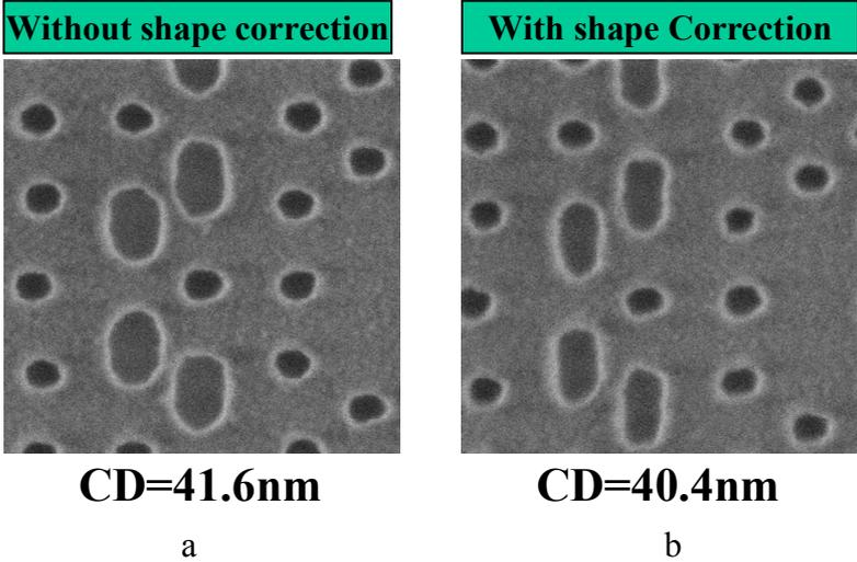
Figure 8 : 32nm contact hole structures patterned at 40nm without (a) and with (b) shape correction
