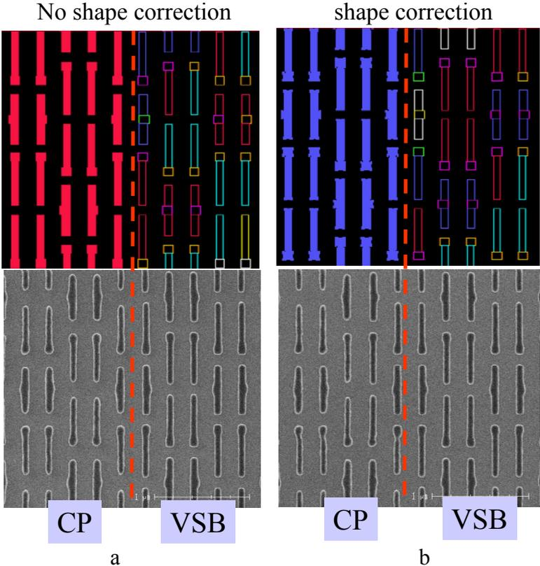
Figure 6 : Comparison of the 65nm SRAM structures obtained without (a) and with shape correction (b)
