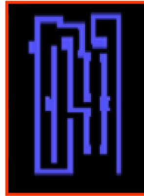
Figure 2 : Example of circuit portion projected by cell projection concept
