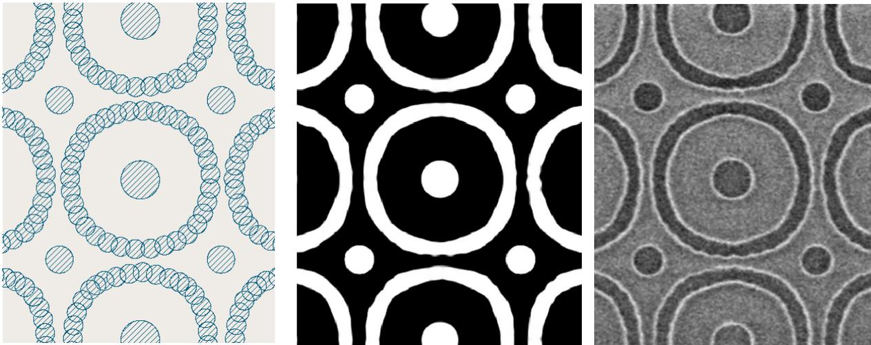
Figure 3. MB-MDP results for 350 nm pitch contacts (pattern C0-1) using overlapping circular shots (left), simulated e-beam mask image (center), and the corresponding mask SEM image (right).
