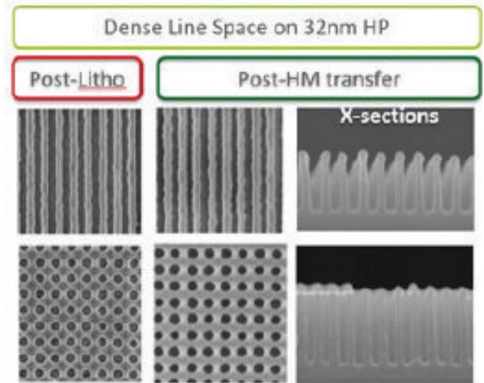
**FIGURE 8.** First imaging performance of the FLX-1200 on full 300mm wafer
