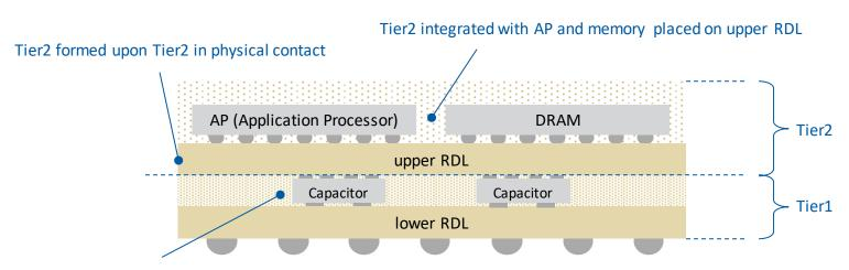
Tier1 integrated with capactiors placed on lower RDL
